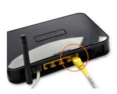
You can connect your computer to your router via the Yellow Ethernet Cable that was you can connect your computer to your router via the Yellow Ethernet Cable that was supplied with the router or if you have a computer or wireless device which already has been connected or paired to your router you can use that.
